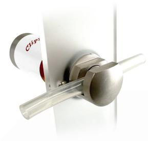
This powerful pinch valve provides the same functionality as Clippard's standard NPV series but with the added benefits of a longer stroke. This makes it ideal for applications that require greater flow or those that utilize viscous or particulate-laden media. As with all Clippard pinch valves, each valve comes pre-installed with 12" (30 cm) of your choice of standard medical/laboratory grade or sanitary food grade silicone tubing.
